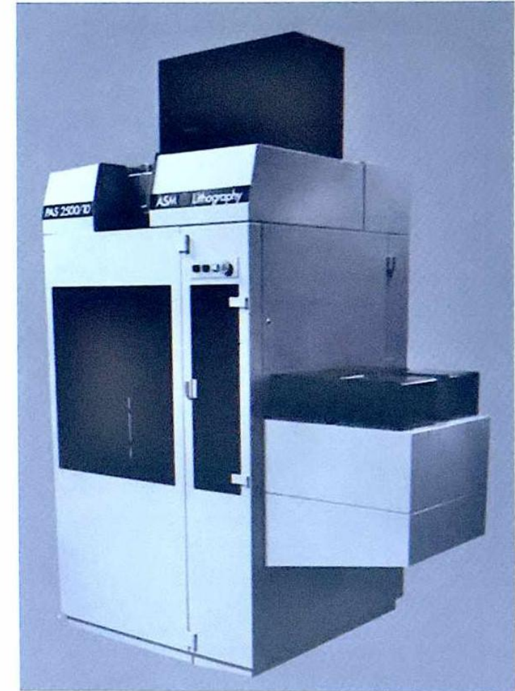
ASML PAS 2500/10 wafer stepper Field size = 20 mm in diameter
